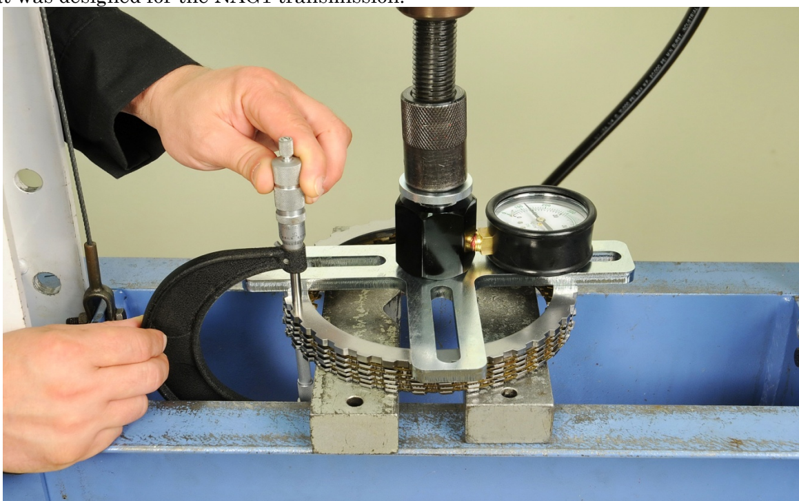
Figure 15: Clutch Pack Height Is Measured After Being Compressed
