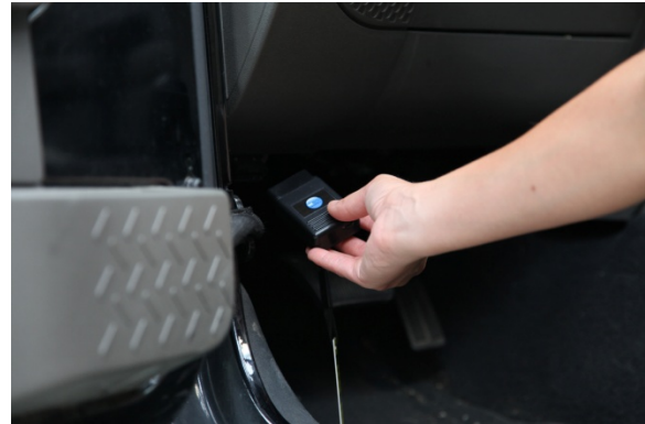
Figure 25: microPod Plugs into the OBDII Port
