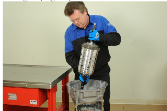
Figure 12: The Gear Train Must Be Removed Vertically
