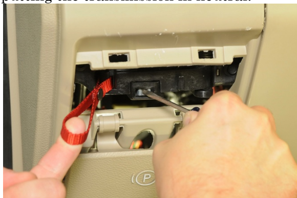
Figure 8: Slide the Lock to Release the Park Release Lever
