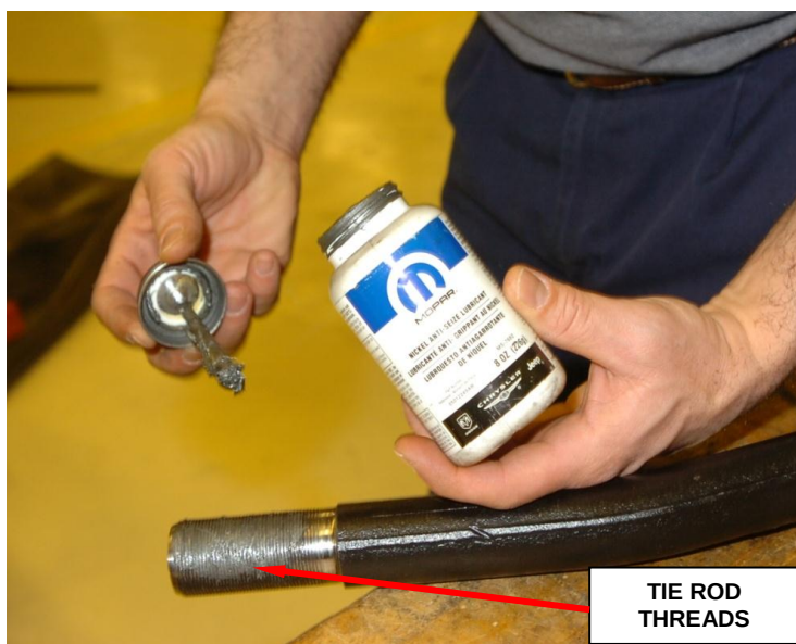
Figure 7 – Apply Light Coat of Anti-Seize
